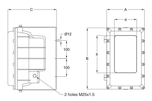
SLEE-40 floodlight kits with 400 W ballast are supplied as standard with a separate enclosure housing starter and capacitor.
